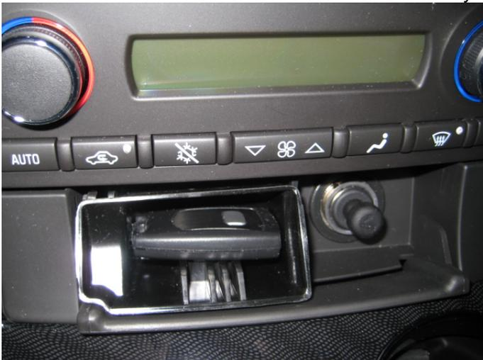
All you do is push the button to open the exhaust, push it again to put it in normal mode. The transmitter has its own battery, just like a typical remote fob.
